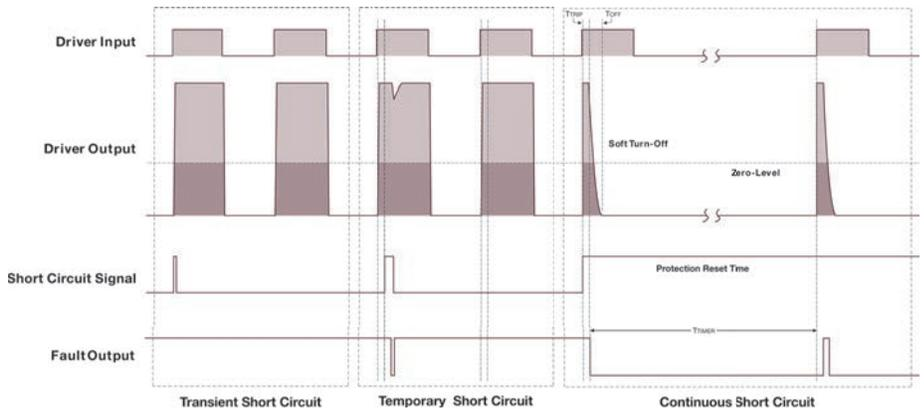
In block two, a temporary short circuit condition extends past the  $T_{TRIP}$  limit (>2.32  $\mu$ s) and triggers a shutdown. When an actual short circuit is detected (at the end of  $T_{TRIP}$ ), the driver provides a soft shutdown. This will limit the transient voltage surge that occurs when large short circuit currents are interrupted. The default soft shutdown time is 5.0  $\mu$ s, which should work for most applications.
