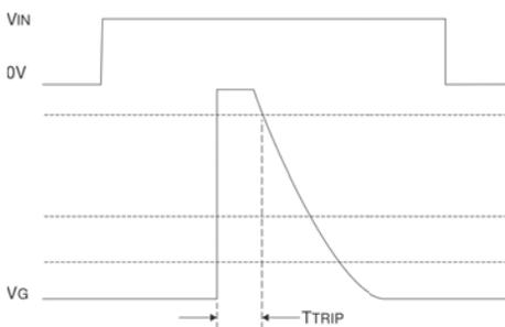
The  $T_{TRIP}$  and fault detection waveforms above illustrate the response of the IGD962-8A to typical fault conditions. In the first block, an instantaneous or transient short circuit occurs.
